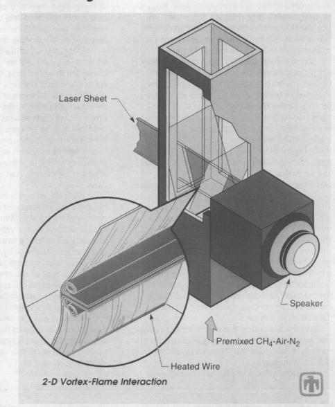
DIAGRAM SHOWS the experimental apparatus used to study the interaction of a vortex with a premixed methane-air flat flame.
